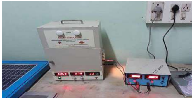
Fig 2: Experimental setup for studying I-V characteristic of Si solar cell
